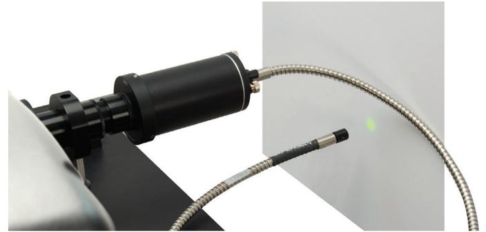
The 77776 in the table below transmits the broad wavelength range of the TLS130B and optically focuses this light output onto one of the Oriel Light Guides or Fiber Bundles.
