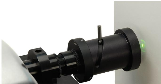
The parts in the table below can be used to mount additional optical components such as Lenses and Filters.
